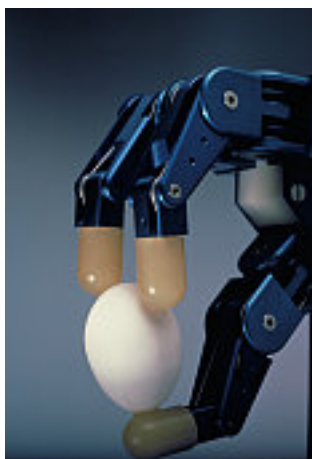
Figure 1.1: The Salisbury Hand, an anthropomorphic robotic hand which uses nine actuators [7]
